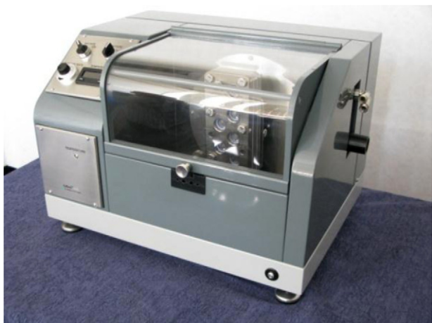
Fig. 4 – ACR mounted in the shaking platform.
