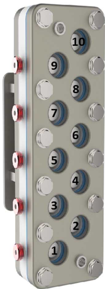
Figure 2. Reaction block from the agitated cell reactor 6 with numbered CSTRs.
