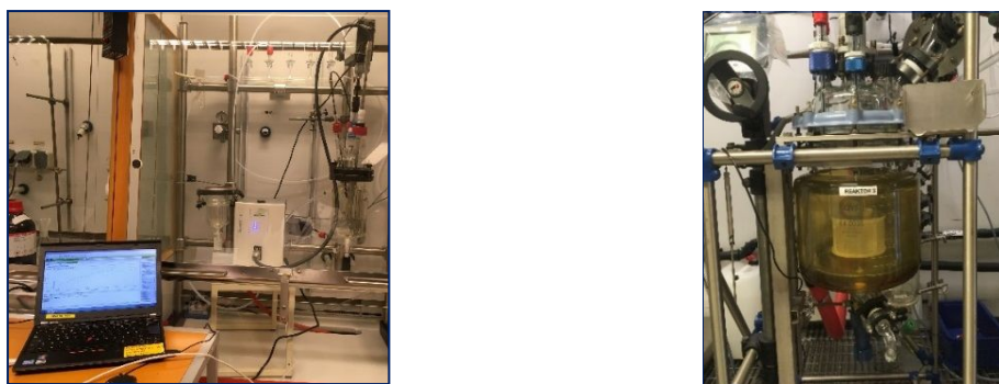
Figure 6: (Left) Reactor setup with in-line FT-IR monitoring and (Right) Reactor set-up for 10 L.
