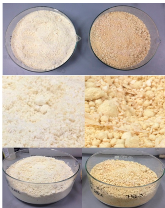
Figure 2. Qualitative comparisons among the particulates produced in flow (left) and in batch (right).
